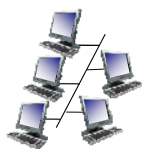
shared wire (e.g., cabled Ethernet)
