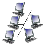
shared wire (e.g., cabled Ethernet)
